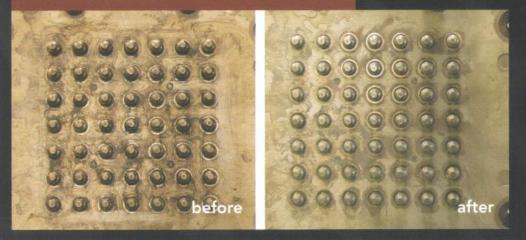
Deburring metal parts with Maxi-Blast plastic media is a unique and effective application. Many zinc and aluminum die castings require only light deburring without affecting the part surface; Multi-Blast (MB), PC and PA media work well for this non-abrasive deburring. Also, machined metal parts have loose burrs that can easily be blasted away without affecting the surface.
