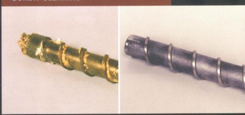
Extrusion, injection and even twin screw cleaning can be done without harsh chemicals or long hours of hand cleaning. Our effective blasting media, used in conjunction with the Maxi-Blast Mobile Screw Cleaning System, reduces cleaning time to an average of 30 minutes per screw.
