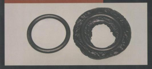
In the cryogenic shot-blast deflashing process, our patented cryogenic grade polycarbonate media (CG) is blasted at rubber parts by means of a turbine blast wheel that spins at speeds of up to 6,000-10,000 RPM. The media impacts with the parts (frozen by means of liquid nitrogen) which are tumbled in the blast machine. Temperatures can reach -300° F (-184° C), effectively freezing the flash, or the excess where the mold halves meet, which is created during the rubber molding process.
