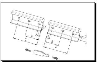
Note: Ferrules have to be used only if the rail web hole is  $\varnothing$  33 mm.
