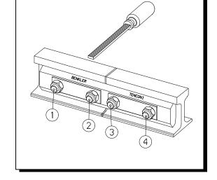
a) One month after installation the nuts must be retightened using the above indicated torque value.
